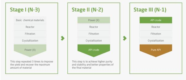
Figure 1: API manufacturing stages
